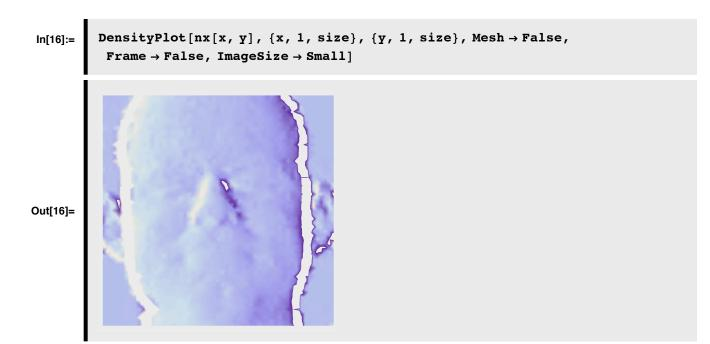
As we saw for intensity, we can also make a plot of the magnitude of the gradient:
